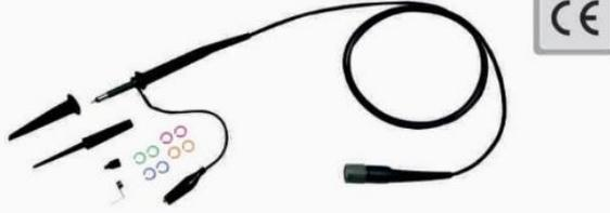
The GTP-200B-4 is a passive high impedance oscilloscope probe designed and calibrated for use on instrument having an input impedance of  $1M\Omega$  shunted by 20pF. However, it may be compensated for use with instruments having an input capacitance of 5~30pF. The probe incorporates a two position slide switch in the head which selects attenuation of x1, x10 position.
