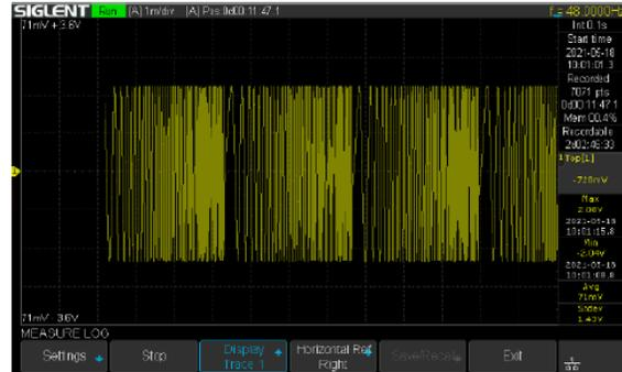
The measurement Logger is designed to collect measurement values for a long time. The data is logged in memory. After logging is complete, the data can be saved into the internal flash or external U disk.
